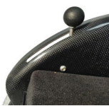
Brakes in side guards, OFF position
